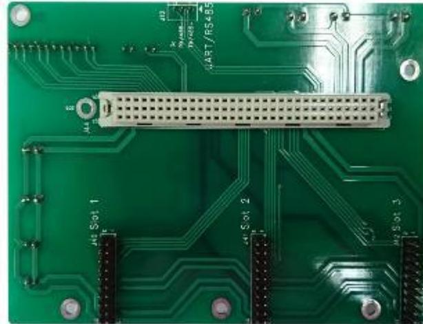
1. Slot: 4 (For three output modules and one control module.)
